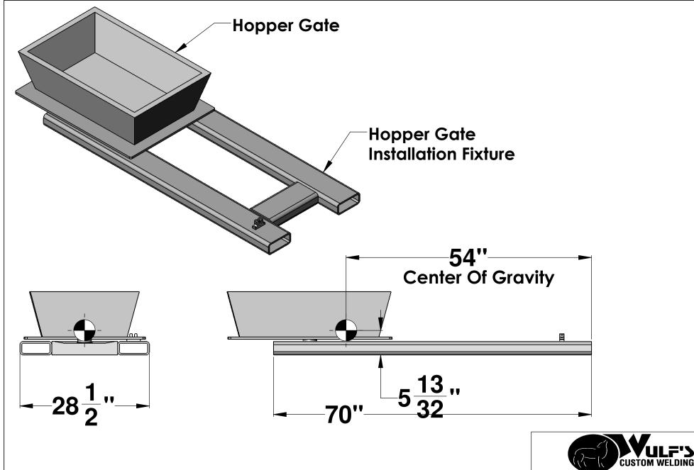
Hopper Gate Installation Fixture 450 Lbs Hopper Gate Maximum Weight 600 Lbs. Total Weight 1050 LBS
