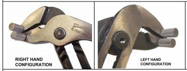
The clamping tines are not tightened when the pliers are shipped to allow transition between right and left handed applications. Tighten the tines after the desired configuration if attained. Right and left hand configurations are shown.
