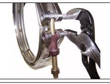
Adjust the pliers channel for the clamping operation. The second or third channel usually works the best for clamp closure. Open the pliers and place the clamping tines in the upper and lower portions of the exhaust clamp band.
