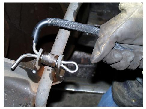
Capacity: Use to bend the legs on any 3/8" or 1/2" diameter cotter pins.
