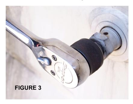
5. When testing is completed, turn the ratchet clockwise to tighten the pet cock.
