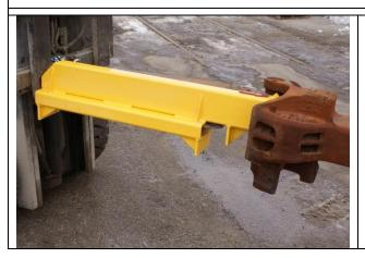
Release the safety chain and place the carrier back into its proper place of storage. Inspect the carrier components again for possible damage.
