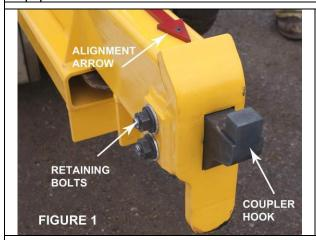
Inspect the carrier prior to use. The safety chain and grab hook must be in place. Check the coupler lifting hook for cracks or excessive wear. The hook retaining bolts must be in place and securely tightened. The part number for a replacement hook is 295-1.
