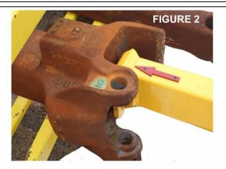
Move the forklift and carrier to the coupler requiring transport. Align the red arrow with the casting hole on the coupler face. Tilt the forklift mast as necessary to ensure the coupler face is as close to parallel with the face of the coupler hook. Move the carrier into the coupler casting hole and apply upward pressure with the forklift mast.
