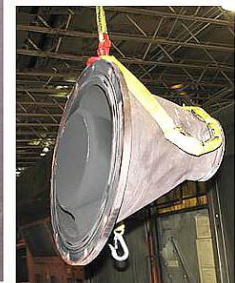
Transition Section Lifter Lifts GEVO Stage 1, Stage 2 & FDL Transition sections. Item # 0570
